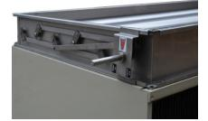
Block casing made from 20 mm polypropylene plates, with plastic composite corner profiles. These are reinforced with fully encapsulated stainless steel profiles. With integral bypass enclosure and aluminium bypass damper. Bypass damper also available on request in stainless steel or plastic.
