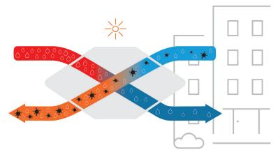
Humidity transfer. With the special Polymer-Membrane both humidity and heat are transferred from return air to supply air. Indoor air quality is therefore greatly increased.
